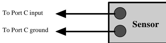
When the sensor is dry, it will be electrically "open". This causes the input port to stay high (its normal state). When the sensor gets wet, its resistance decreases and the input port will go low (to ground).
